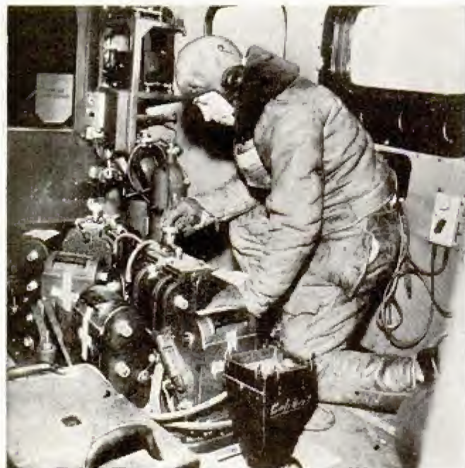
Here one of the army's multi-lens cameras is installed in a plane to shoot through the floor, mapping the country by strips
